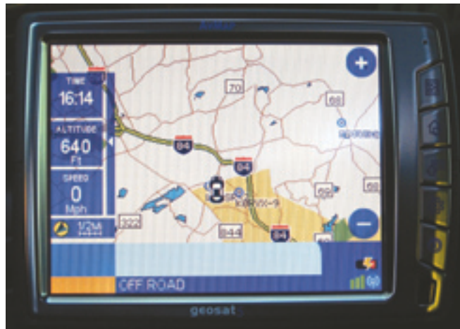
Figure 2 — The G5's map shows APRS station data received from the Kenwood TM-D710A near the center of the display. The blue area near the bottom of the screen is for location and driving directions when the vehicle is in motion.
